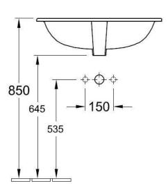
PRODUCT NO: **41625001**, O.novo Under-Counter Basin **OD** 580x370mm (**ID** 530x320mm) Recommended overflow waste - code 94238 Overflow hole should be positioned to the front of the cabinet
